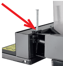
Fig. 4: Axis of rotation of the actuation arm 8 t wood splitter
