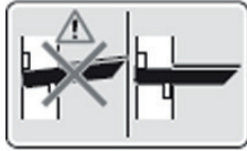
Fig. 9: Attach splitting table correctly
