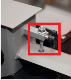
Fig. 11: Star grip screw on the switching rod, 7 t wood splitter
