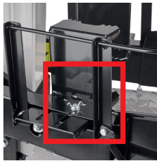
Fig. 10: Wing screw on the wood clamp
