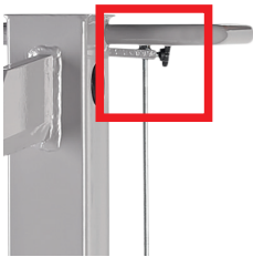
Fig. 12: Star grip screw on the switching rod, 8 t wood splitter
