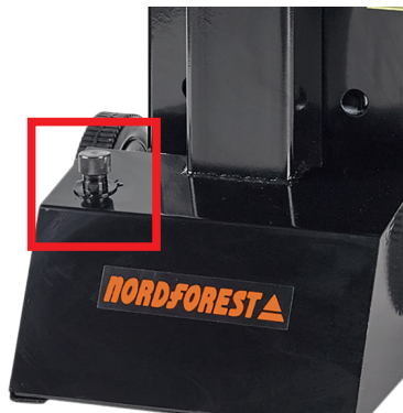
Fig. 19: Filling screw with dipstick, 8 t wood splitter
