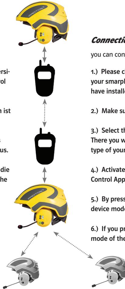
**Connection with an additional bluetooth device, e.g. radio device**
