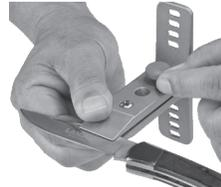
**PRO TIP:** For best results, the gap at the back of the clamp should be equal or *slightly* greater than the gap near the front jaws of the clamp. Approx. 5/8" of the blade should be exposed from the end of the clamp. *If the hone hits the thumbscrew, replace it with the flat head screw provided.* For blades approx. 1/2" and under wide, use the notch in the clamp. Position average or oversized blades beyond notch and well into the knife clamp (see diagram).
