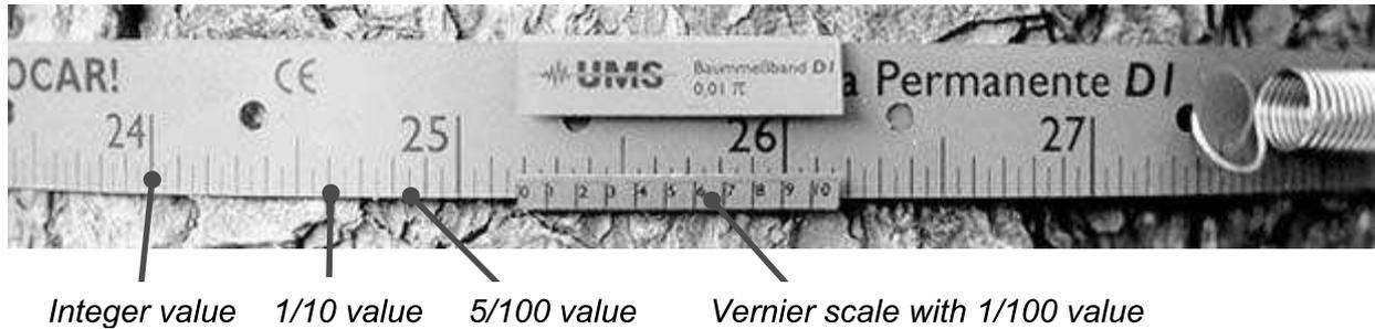
On the band, the numbered lines are the integer value. The longer of the short lines is the 1/10 value, and the shortest line is the 5/100 value. On the vernier scale you can read the 1/100 value.
