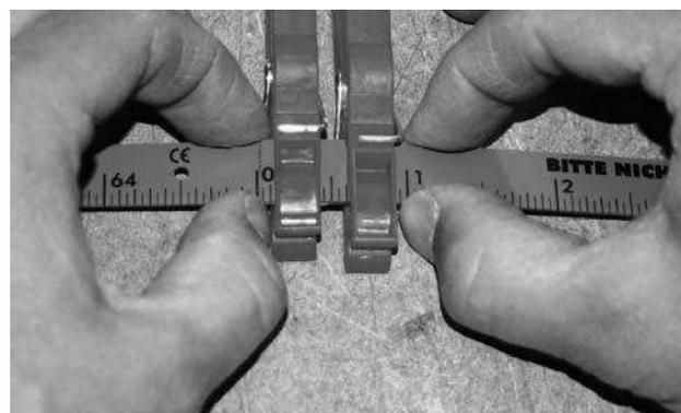
3, Check the result and cut off overlaying remains of the adhesive.
