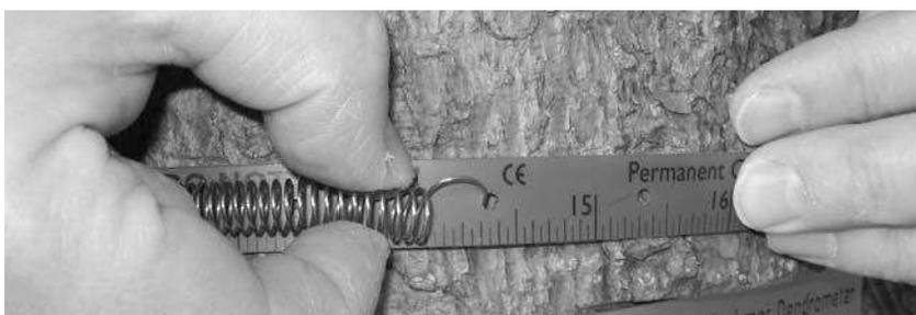
The other end of the spring is attached to the tied around band with a spring excursion of 30mm (60mm). The spring's tension then is approx. 0.2N.
