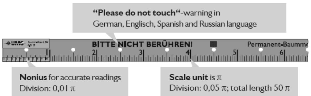
An exceptional feature of this girth tape is the minimised friction. There is only a printing on the top side to reduce the friction between the backside and the bark. The vernier is specially shaped for a frictionless guidance and the eyelets are manufactured without burr.
