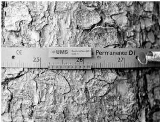
The installation is easy and quick. Lead the loose end of the tape-measure around the trunk and through the vernier. Then, hook in the spring to one of the eyelets with an initial spring expansion of min. 2 cm.
