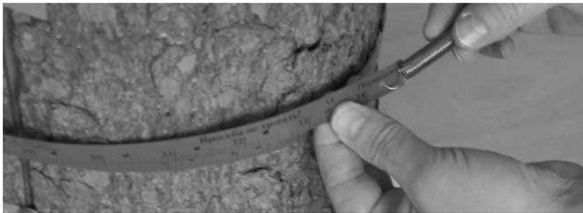
Tighten the band and hook the spring into one of the 3 last eyelets.
