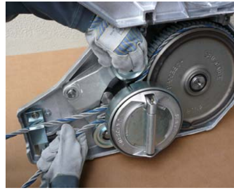
HIT-TRAC 16 B Inserting the rope, See Chapter 5.2
